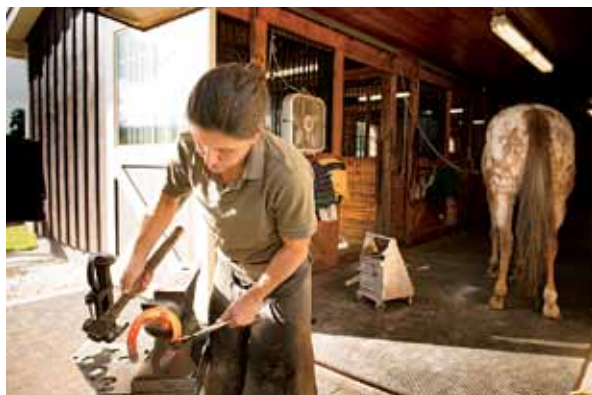
Hammering the orange-hot shoe requires less brawn, and more finesse, than many imagine. With her mobile blacksmith shop (left) parked at the barn door, Cloos grinds a bevel onto Willoughby's shoe as he stands by.
