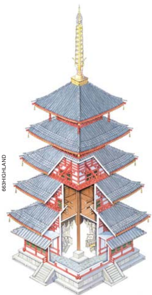
Left: A grove of cypress trees prepared for harvest. Above, left: Built in 607, Horyuji monastery is Japan's oldest surviving example of monumental timber-frame architecture. Its five-story pagoda (top) enshrines relics of the Buddha. The pagoda's main structural element, pictured in the cutaway (right), is its heart pillar, a single cypress tree that keeps the building steady during earthquakes. Above, right: More cypress pillars hold up the monastery's outer ring and main hall.
