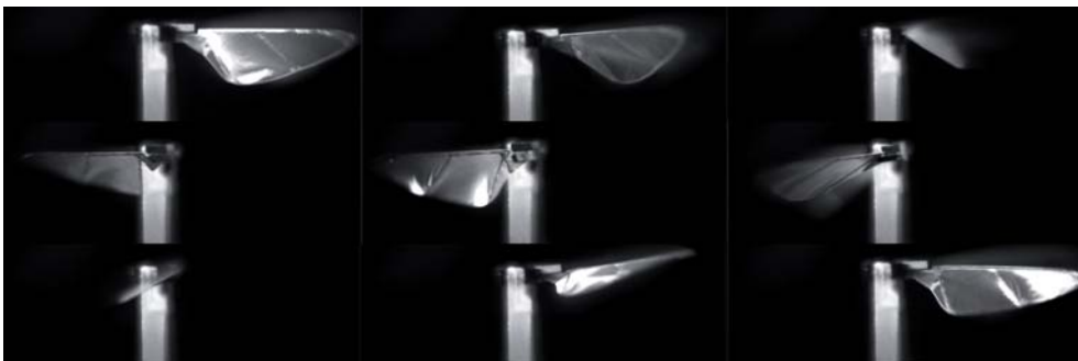
The fly's wings, made of polymers that respond to an electric current, flap and rotate like those of a real fly, beating 120 times per second.
