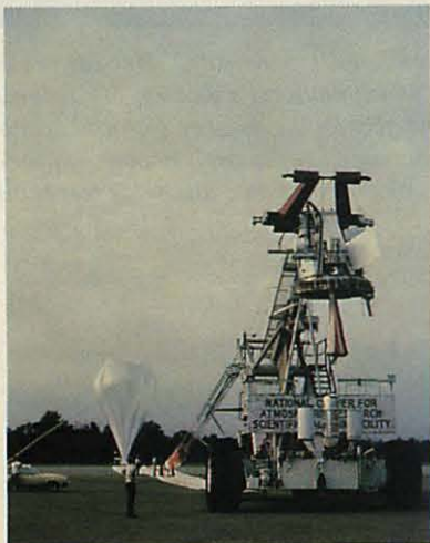
The reel-down launch. The spool truck with the balloon's upper end looped over its spool (above) and partially inflated (right). Bottom, from left to right, the entire balloon-payload assembly; the balloon rising behind Tiny Tim; the balloon's attachment cables approaching the vertical. Opposite, the entire rig, which at 800 feet stands taller than Boston's John Hancock Tower, at its moment of release.
