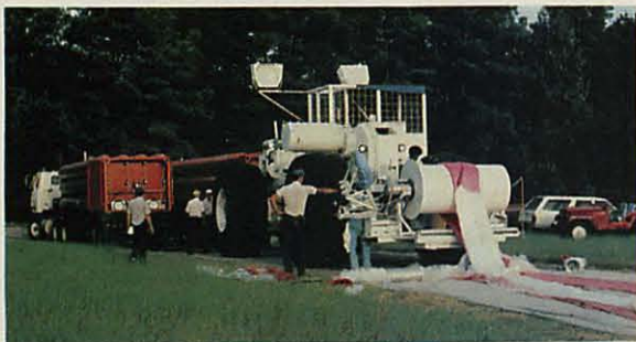
The reel-down launch. The spool truck with the balloon's upper end looped over its spool (above) and partially inflated (right). Bottom, from left to right, the entire balloon-payload assembly; the balloon rising behind Tiny Tim; the balloon's attachment cables approaching the vertical. Opposite, the entire rig, which at 800 feet stands taller than Boston's John Hancock Tower, at its moment of release.
