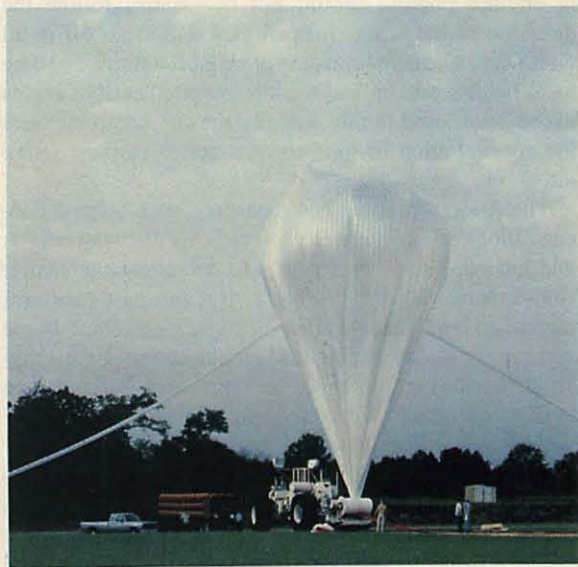
The reel-down launch. The spool truck with the balloon's upper end looped over its spool (above) and partially inflated (right). Bottom, from left to right, the entire balloon-payload assembly; the balloon rising behind Tiny Tim; the balloon's attachment cables approaching the vertical. Opposite, the entire rig, which at 800 feet stands taller than Boston's John Hancock Tower, at its moment of release.
