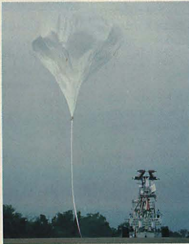
The reel-down launch. The spool truck with the balloon's upper end looped over its spool (above) and partially inflated (right). Bottom, from left to right, the entire balloon-payload assembly; the balloon rising behind Tiny Tim; the balloon's attachment cables approaching the vertical. Opposite, the entire rig, which at 800 feet stands taller than Boston's John Hancock Tower, at its moment of release.
