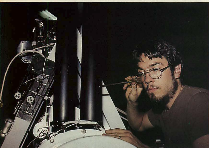
Craig Schiller listens, via the winch platform's black stacks and a screwdriver, to noises made by the winch motor bearings.
